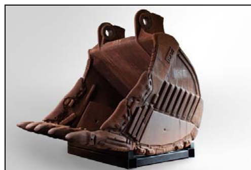
The rock shovel bucket measures nearly three metres high and is made of solid steel, weighing 15.2 tonnes. Photo: Jason McCarthy, National Museum of Australia.
